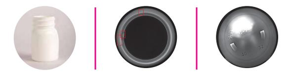
Optomech BIS is a high performance system for checking the visual defects in plastic injection blow moulded bottles
